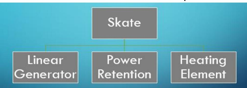
The three subsystems involved in the system are shown in the block diagram above. The linear generator harvests the energy needed, which is then stored in the power retention system and put into the heating element to raise the temperature of the blade. These subsystems are placed within the TUUK of the skate and are connected through circuitry. The heating element will sit on the blade to ensure for reliable heat transfer.
