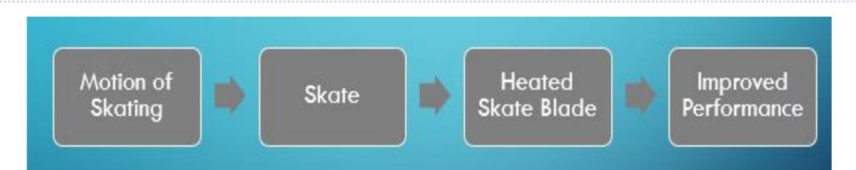
The system uses the motion of the player's skates to harness energy through Faraday's Law of induction. Once the energy is harvested it is used to transfer heat from the circuitry to the blade. When the blade reaches the desired temperature of 41°F the performance of the player is improved by standards that meet Thermablade's product.
