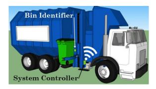
Figure 3 - Household waste tracking system retro fitted to waste reception vehicle
