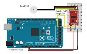
Figure 9 - Load cell & A/D amplifier wiring diagram
