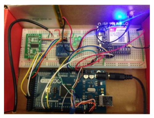
Figure 7 - Constructed device inside enclosure
