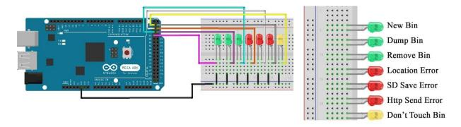
Figure 12 - LED wiring Diagram (LEDs not shown)
