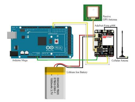
Figure 11 - Adafruit Fona 808, GSM board Battery, GPS & Cellular Antennas wiring diagram In addition to the main devices of the system, there is one method of user interaction that is a part of the hardware. As the system progresses through a routine waste reception, there is a series of seven LEDs that notify the operator of the status of the system. Not shown in the figures below are the resistors required to lower the current flowing through the resistors.
