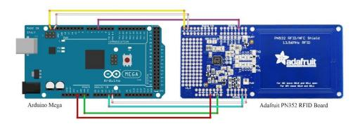
Figure 8 - RFID reader/write board wiring diagram
