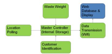
Figure 5 - Initial top-level function block diagram
