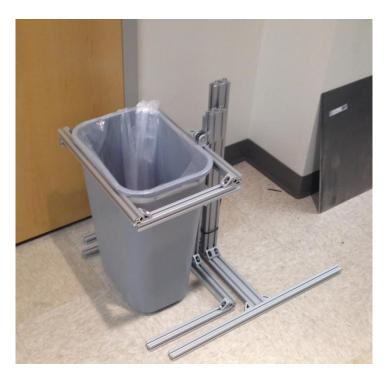
Figure 29 - Full bin on rig, establishing full weight
