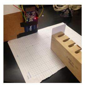
Figure 23 - RFID testing using a parallel tag orientation
