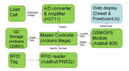
Figure 6 - Top level devices and connectivity block diagram
