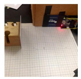
Figure 22 - RFID testing using a perpendicular tag orientation
