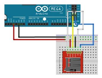
Figure 10 - Micro SD card board wiring diagram (pull-up and pull-down resistors)
