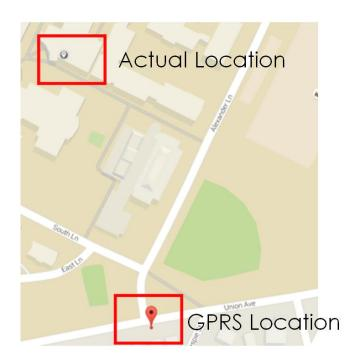
Figure 25 - GPRS location test results in comparison to actual location 204 meters away Although the data is not accurate enough to use to verify the identity of a bin collection, this result could still be relevant in assessing waste trends.
