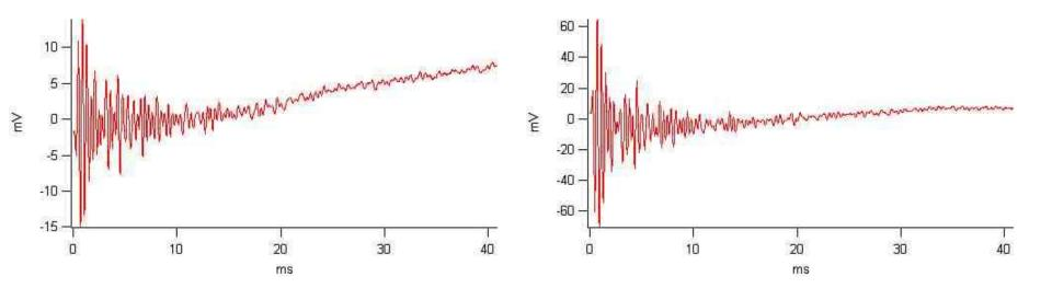
Shown (left): deflection impulse response to a 4V discrete voltage change to z piezo
