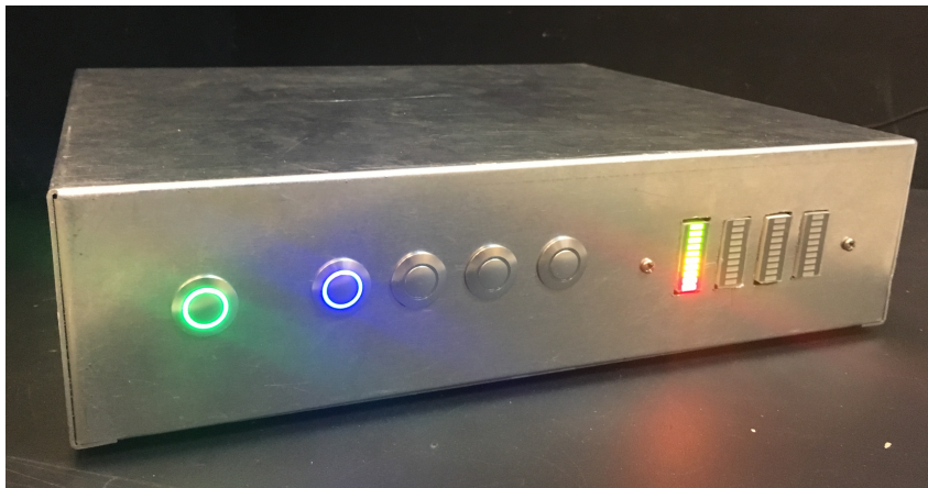
Figure 11: Completed Device Exterior Front. Shows, from left to right, power button, four selection buttons, and four bar LED indicators corresponding to selection buttons.
