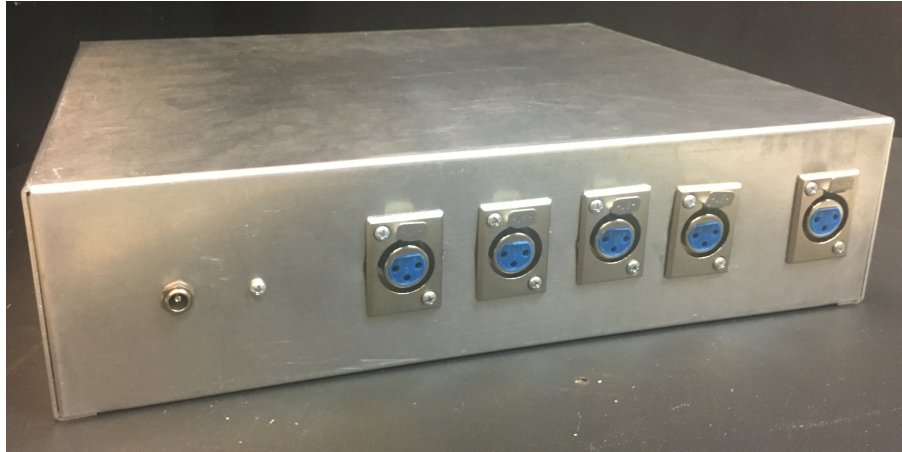
Figure 12: Completed Device Exterior Back. Shows, from left to right, power input, four XLR microphone inputs, one XLR microphone reference input.
