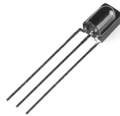
Figure 11: TSOP 38238 IR receiver.[13]
