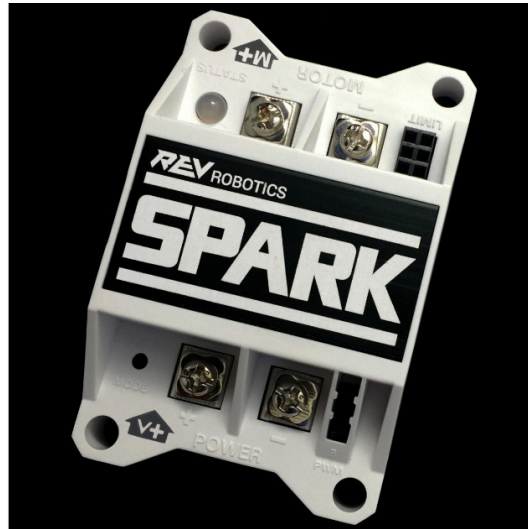
Figure 25: Close up of the Motor Controller.
