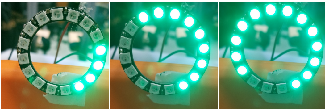
Figure 37: Tail light NeoPixel's LEDs incrementally be lit up when device is accelerating forward.
