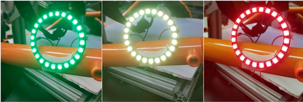
Figure 35: Three stages of battery level shown on a 24 LED NeoPixel Ring.
