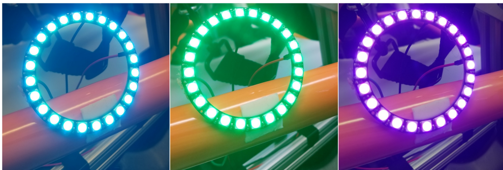
Figure 36: Three different speed profiles shown on a 24 LED NeoPixel Ring.
