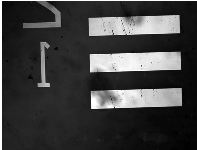
USAF Resolution Test Chart Group 2 Element 1
