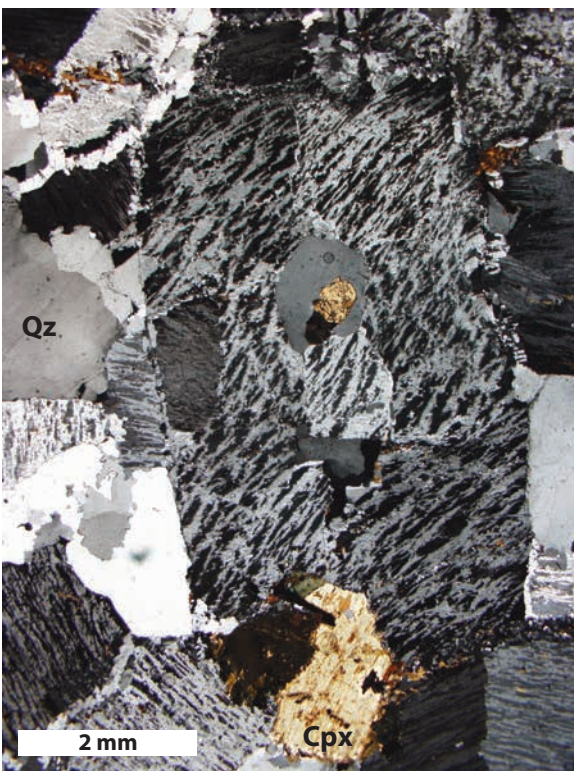
Figure 21. A photomicrograph of the Cape Ann granite in crossed-polarized light showing the micropertthite texture. Quartz (Qz) and aegirine-augite (Cpx) are also visible.
