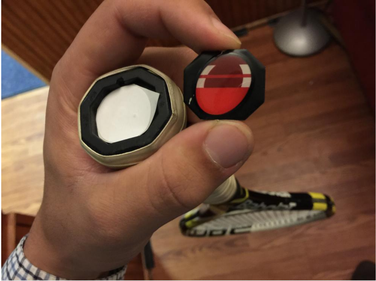
Figure 6. Tennis Racket with NFC Tag installed
